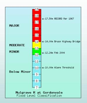
Continuous comparison of rain & river data to threshold values
